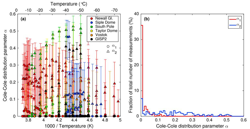
**Figure C1.** (a) Temperature dependence of  $\alpha$  for the fastest two relaxations (two lowest values of  $\tau$ ) in the Greenland and Antarctic ice cores studied by *Stillman et al.* [2013a]. Circles represent the fastest relaxation ( $j = 1$  in equation (C1)) and triangles represent the second fastest ( $j = 2$ ). Error bars represent the 95% confidence intervals for each value where available. (b) Distribution of inferred values of  $\alpha_1$  and  $\alpha_2$ .
