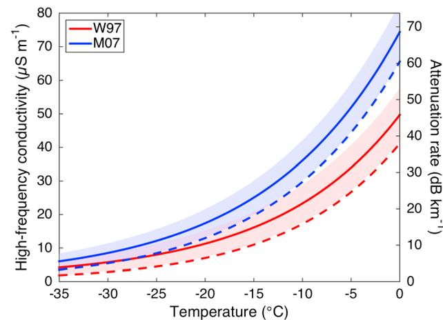
**Figure 3.** HF-limit ice conductivity  $\sigma_{\infty}$  as a function of the likely temperature range of the GrIS, using two different  $\sigma_{\infty}$  models (Table 2). Solid lines and shading (uncertainty) are calculated using the mean and standard deviation of impurity concentrations during the Holocene from the GRIP ice core. Dashed lines are calculated using mean LGP impurity concentrations.
