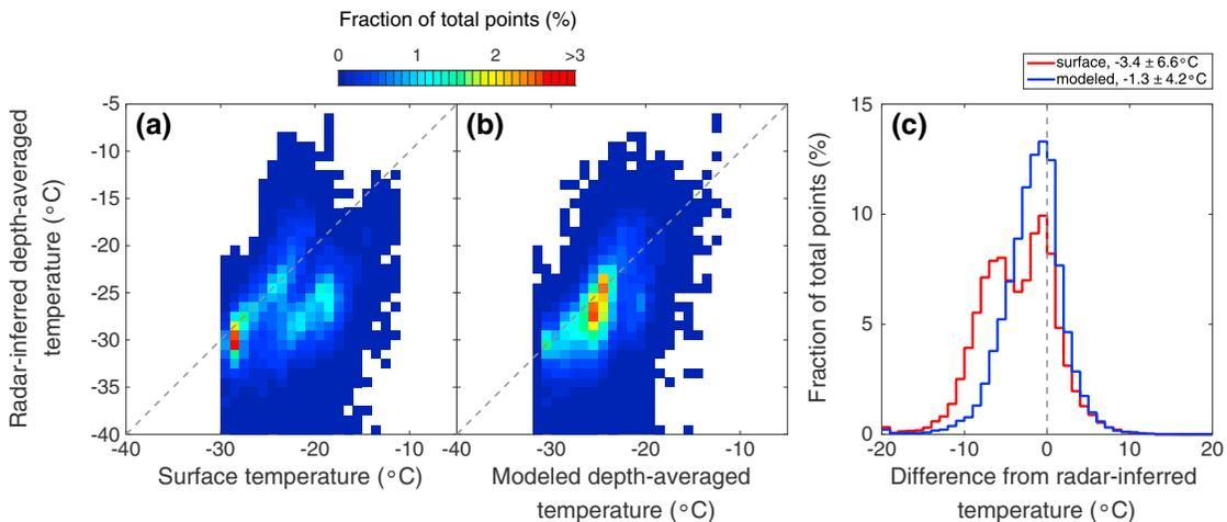
**Figure 9.** (a, b) Relationships between  $T_s$ ,  $\bar{T}_m$ , and  $\bar{T}_a$ . (c) Distribution of values of  $\Delta T_s$  (red) and  $\Delta T_m$  (blue). Legend gives best-fit mean and standard deviation for a Gaussian distribution.
